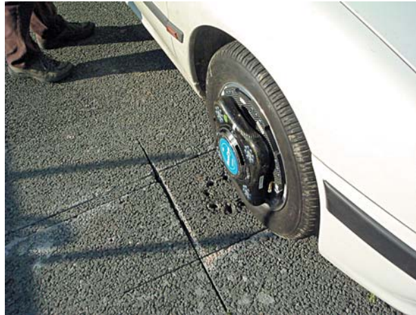
figure 1 The Kistler wheel on the MEVI system
