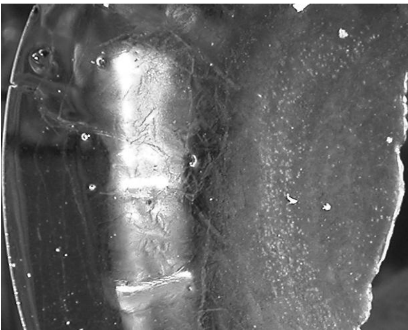
Figure 2. Ice scale layer formed on the scraped heat exchanger surface. The left transparent area corresponds to the outer area near the wall of the crystallizer. In the middle area the ice is not transparent and softer.
