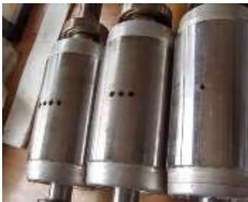
Fig.7. Broken bars
