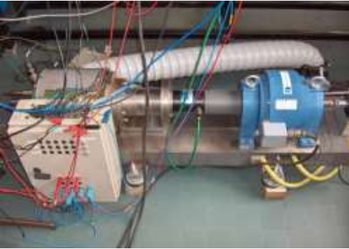
Fig.6. Test bench of induction motor
