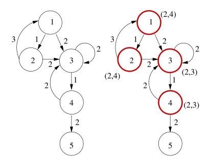
Fig. 1. (a) an example graph (b) the graph annotated with critical nodes and critical cycles  $% \left( \mathbf{x}^{\prime}\right) =\left( \mathbf{x}^{\prime}\right) \left( \mathbf{x}^{\prime}\right) \left($
