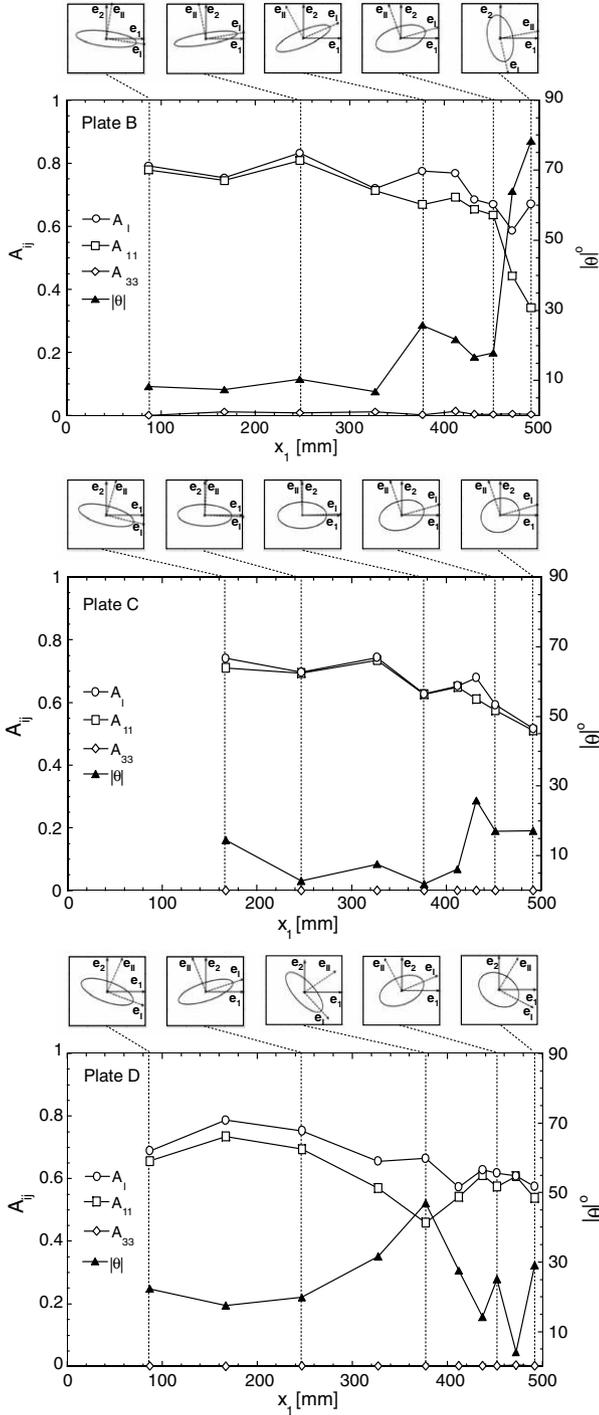
Fig. 9. Evolution of the components  $A_{11}$ ,  $A_{33}$  and  $A_7$  of the orientation tensor and the absolute value of the angle  $|\theta|$  between the major principal vector  $e_1$  and the flow direction  $e_1$ , for compression moulded plates B, C and D.
