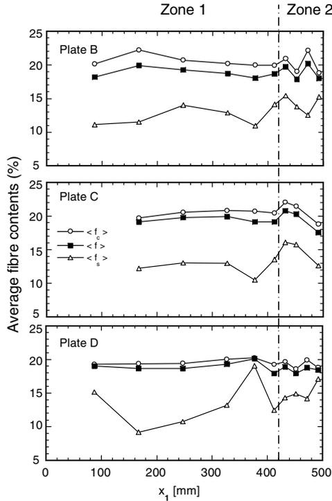
Fig. 5. Evolution of the average values of the fibre contents  $\langle f_c \rangle$ ,  $\langle f_s \rangle$ ,  $\langle f \rangle$  along the flow direction  $x_1$  of compression moulded plates B, C and D.
