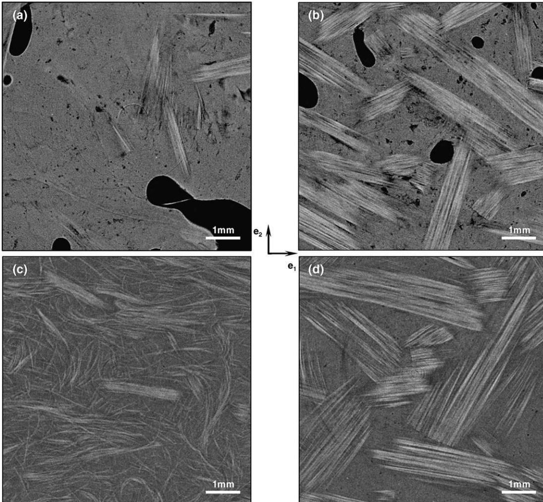
Fig. 7. 2D micrographs of the non-deformed sample A (a and b) and a compression moulded sample B<sub>4</sub> (c and d), close to the skin ((a and c),  $x_3 = 0.02$  mm) and in the middle of samples ((b and d),  $x_3 = h/2$ ).
