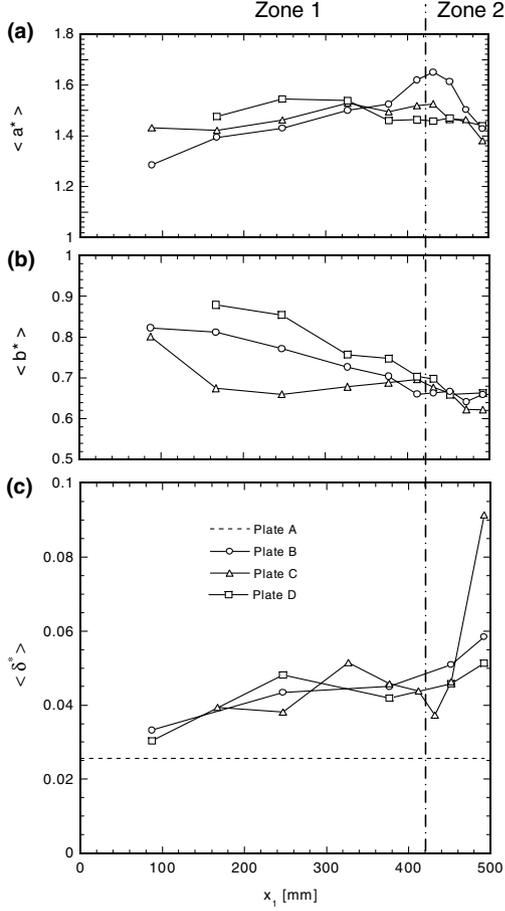
Fig. 8. Evolution of the dimensionless width  $\langle a^* \rangle$  (a) and thickness  $\langle b^* \rangle$  (b) of the bundles, as well as the dimensionless deflection of bundles  $\langle \delta^* \rangle$  (c) in core zones and along the flow direction  $x_1$  of compression moulded plates B, C and D.
