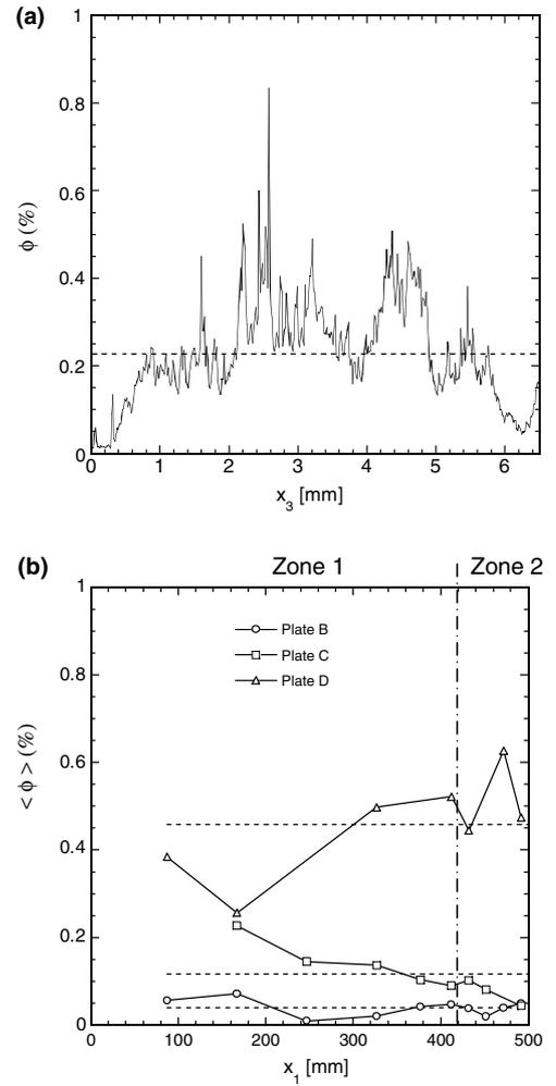
Fig. 6. Evolution (a) of the porosity  $\phi$  through the thickness  $x_3$  of the deformed sample  $C_2$  and (b) of the average porosity  $\langle \phi \rangle$  along the flow direction  $x_1$  of compression moulded plates B, C and D.
