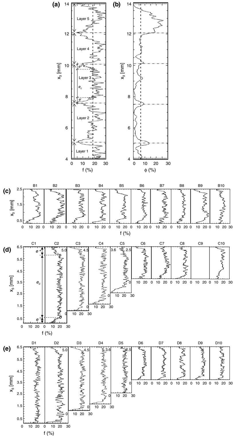
Fig. 4. Evolution (a) of the fibre volume fraction  $f$  and (b) of the porosity  $\phi$  through the thickness  $x_3$  of the non-deformed sample A. Evolution of the fibre volume fraction  $f$  through the thickness  $x_3$  of the samples cut from plates B (c), C (d) and D (e).
