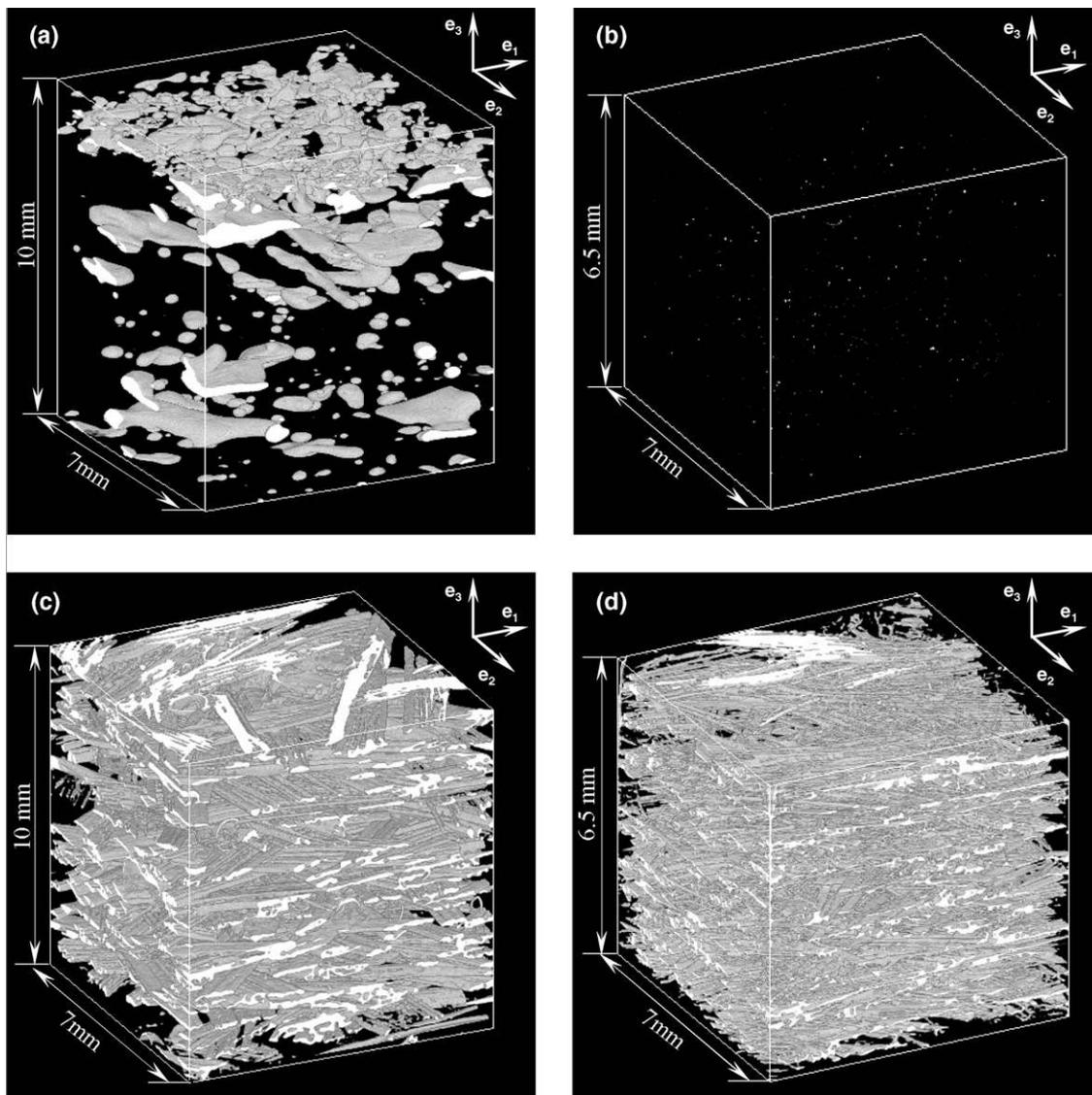
Fig. 3. 3D micrographs taken from samples A (a and c, non-deformed sample,  $0 \text{ mm} < x_3 < 10 \text{ mm}$ ) and C<sub>2</sub> (b and d, after compression moulding,  $0 \text{ mm} < x_3 < 6.5 \text{ mm}$ ), showing the pores (a and b) and the bundles (c and d). They have been obtained by X-ray microtomography with the phase contrast mode, followed by a filtering, a thresholding and a binarisation.
