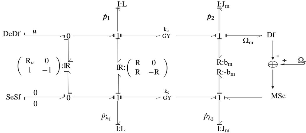
Figure 9. Bond graph representation of the DC motor optimal control problem
