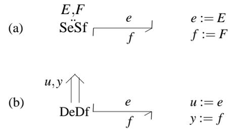
**Figure 11.** (a) Double source, (b) double sensor
