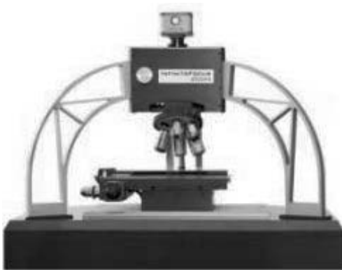
Figure 4. The optical device measurement: InfinitFocus ®
