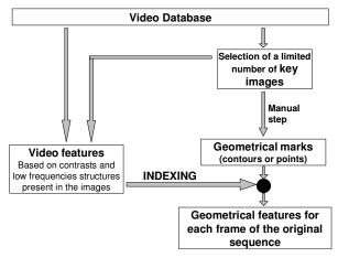
Figure 1: General principle of the retro-marking algorithm.
