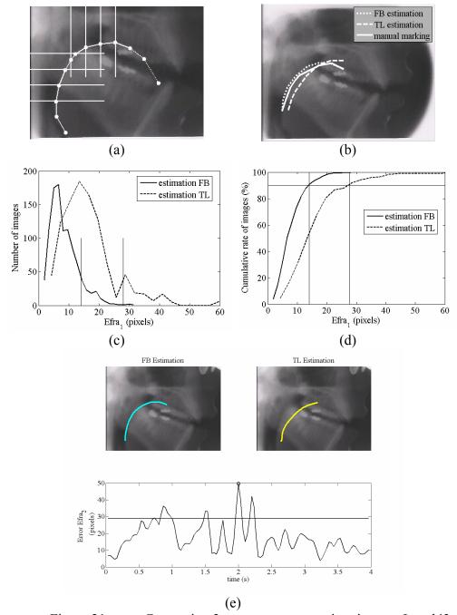
Figure 21: Comparing 2 tongue contour estimations on Laval43 (a) Only 8 *dof* (defined by horizontal and vertical lines) are taken into account in the comparison.
