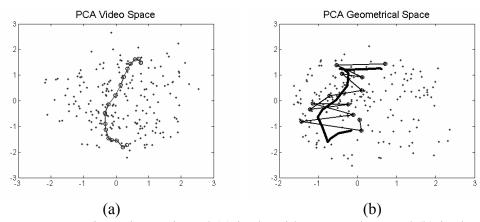
Figure 9: Trajectories projected (a) in the video PCA plane and (b) in the geometrical PCA plane via the indexing (in thin line) and via the 3-neighbor-indexing (in thick line).
