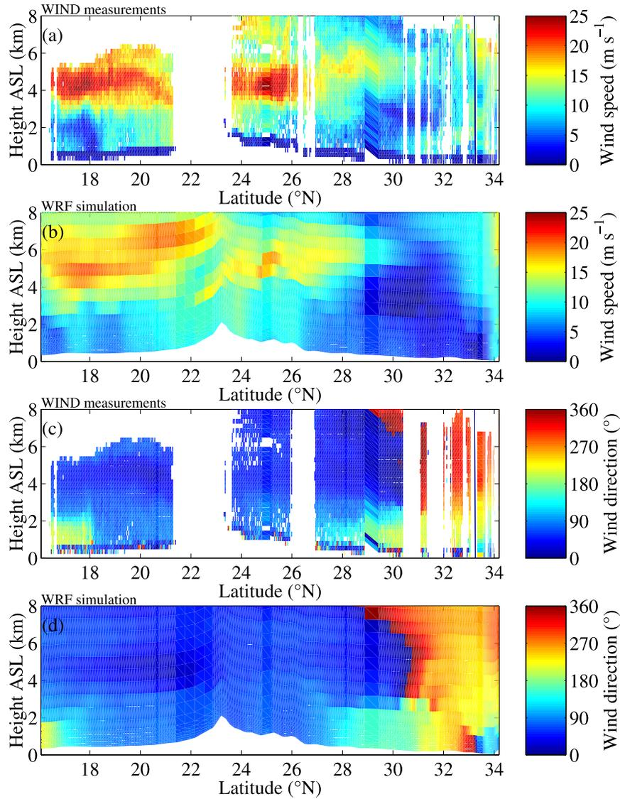
**Figure 11.** Vertical cross section of (a) wind speed and (c) wind direction retrieved from the WIND measurements along the leg flown by the DLR Falcon 20 between 0850 and 1235 UTC (Figure 1) after quality-control and debiasing procedure [Dabas *et al.*, 1998, 1999]. (b and d) Similar to Figures 11a and 11c but corresponding to the simulated data from WRF with 20-km mesh grid resolution.
