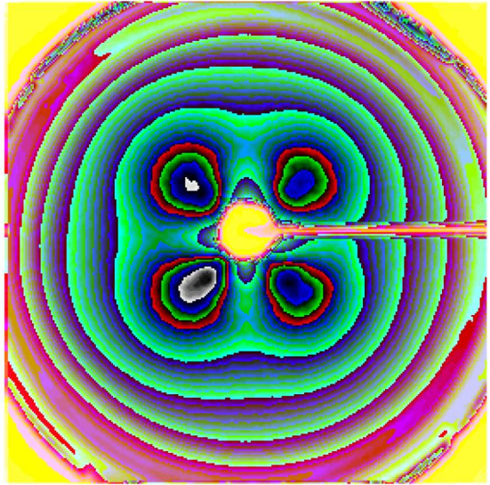
Fig. 2. Contour level image of polarization patterns on the surface of a beaker of a colloidal solution [22] of 2 \mu\text{m} latex beads. Linearly polarized light is incident at a spot at the center of the image. The surface of the beaker is imaged with a camera through a linear analyzer. The analyzer is crossed with respect to the polarization of the incident beam. We see a clear fourfold symmetry in the intensity of the backscattered light with the maximum in inclined intensity at an angle of 45 degrees to the direction of the polarizers.
