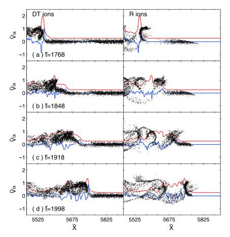
**Figure 13.** Evolution of phase space plots  $\tilde{v}_{ix}$  versus  $\tilde{x}_i$  for (left) DT ions and (right) R ions, and here, the ions have Maxwellian distribution with the initial thermal speed  $0.5\tilde{V}_A$ . The magnetic field  $\tilde{B}_z$  (red line) and electric field  $\tilde{E}_x$  (blue line) are shown in the plots for reference. Results are obtained for the time-reforming shock regime.
