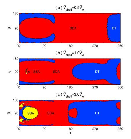
**Figure 5.** The angular domain in  $\phi$ - $\theta$  velocity space for the incident ions undergoing SDA (red), SSA (yellow), and DT (blue) at profile A. (a)  $\tilde{V}_{shell} = 0.5\tilde{V}_{A}$ . (b)  $\tilde{V}_{shell} = 1.0\tilde{V}_{A}$ . (c)  $\tilde{V}_{shell} = 3.0\tilde{V}_{A}$ .
