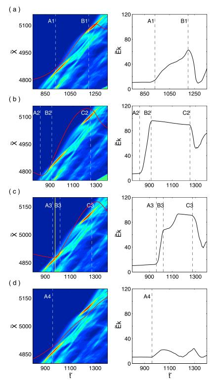
Figure 10. Four typical (left) ion trajectories and (right) kinetic energy versus time for the time-reforming shock regime. The vertical dash lines denote some key points.
