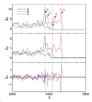
**Figure 2.** Plots of the shock profiles at three typical times. "O" and "N" denote positions of the old and new ramps during one reforming cycle, respectively. (line A,  $\tilde{t} = 1552$ ; line B,  $\tilde{t} = 1600$ ; line C,  $\tilde{t} = 1744$ ). The main ramp location is marked by dashed line for each profile.
