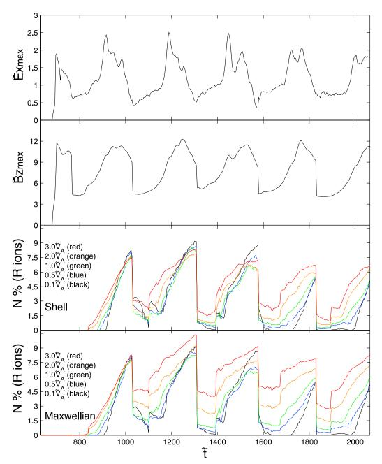
**Figure 14.** Time history of the maximum values of the electrostatic field  $\tilde{E}_{x \max}$  and the magnetic field  $\tilde{B}_{z \max}$  around the shock ramp and of the number of the reflected ions. Results are obtained for different radii (shell distribution) and thermal velocity (Maxwellian distribution), respectively.
