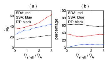
**Figure 12.** (a) The average kinetic energy of SDA (red), SSA (blue), and DT (black) ions in downstream and (b) their percentage as a function of their initial radius of the shell distribution. Results are obtained for the time-reforming shock regime.
