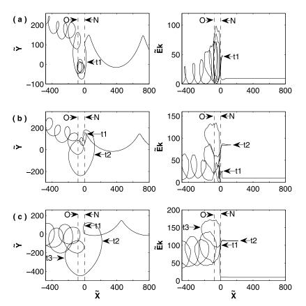
**Figure 7.** Three typical ion orbits and kinetic energy versus  $\tilde{X}$  obtained for shock profile C. Ions suffer from multistage accelerations. Dashed lines "O" and "N" denote the locations of the old and new ramps, respectively.
