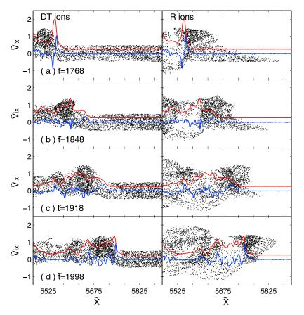
**Figure 9.** Evolution of phase space plots  $\tilde{v}_{ix}$  versus  $\tilde{x}_i$  for (left) DT and (right) R ions for the timereforming shock regime. The initial radius of the shell distribution is  $3.0\tilde{V}_A$ . The magnetic field  $\tilde{B}_z$  (red line) and electric field  $\tilde{E}_x$  (blue line) are shown in the plots for reference.
