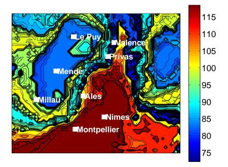
Figure 10: Representation of the pointwise 10 years- return level (in millimeters), estimated with  $\hat{q}^{\pi}$ , as a function of the longitude and latitude.
