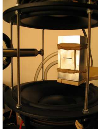
Figure 2: Experimental setup. Jet exit, speakers and acoustic velocity sensor.
