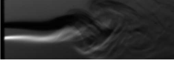
Figure 3: Jet issued from a squared exit, Re: 500 , Jet speed: 7.5 m/s, Excitation freq.: 532 Hz, Str: 0.44 . Visualized with Schlieren technique: the two shear layers appear with opposite light refractive gradient, so that the upper shear layer gets darker while the lower shear layer gets lighter than the average gray level. The jet oscillating movement shows a very small transverse deviation at the beginning of the jet, slowly growing, up the point where the flow rolls up and finally breaks into vortices and later turbulence.
