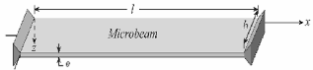
Fig. 2. The clamped-clamped microbeam with dimensions l , h and e .
