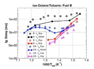
Figure 5: Experimental and simulated main  $(t_{ig})$  and cool flame  $(t_{cf})$  auto-ignition delays for fuel B and iso-octane for pressures between 12 bar and 16.1 bar and Equivalence ratio: 1. Rapid Compression Machine of Vanhove et al. [25].
