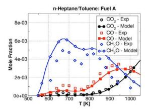
Figure 8: Experimental and simulated mole fractions of  $CO_2$ , CO and  $CH_2O$  as of function of temperature for fuel A. Pressure: 10 bar, Equivalence ratio: 0.2, Residence time=0.5 s. Jet Stirred Reactor of Dubreil et al. [27].
