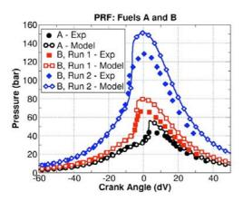
Figure 1: Experimental and simulated pressure curves for fuels A (Run 1) and B (Run 1 and Run 2). Initial temperature and pressure at start of simulations (99° BTDC) – Fuel A/Run 1: 460 K, 1.2 bar, Fuel B/Run 1: 470 K, 1.7 bar, Fuel B/Run 2: 420 K, 3.2 bar. HCCI engine of Andrae et al. [4].
