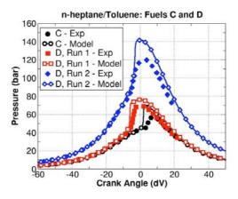
Figure 2: Experimental and simulated pressure curves for fuels C (Run 1) and D (Run 1 and Run 2). Initial temperature and pressure at start of simulations (99° BTDC) – Fuel C/Run 1: 470 K, 1.6 bar, Fuel D/Run 1: 470 K, 1.6 bar, Fuel D/Run 2: 420 K, 3.1 bar. HCCI engine of Andrae et al. [4].
