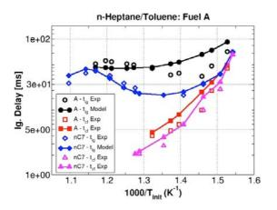
Figure 4: Experimental and simulated main  $(t_{ig})$  and cool flame  $(t_{cf})$  auto-ignition delays for fuel A and n-heptane. Pressures between 3.7 bar and 4.9 bar and Equivalence ratio: 1. Rapid Compression Machine of Vanhove et al. [25].
