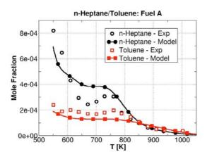
Figure 7: Experimental and simulated mole fractions of n-heptane and toluene as of function of temperature for fuel A. Pressure: 10 bar, Equivalence ratio: 0.2, Residence time=0.5 s. Jet Stirred Reactor of Dubreil et al. [27].
