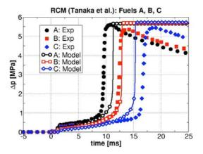
Figure 3: Experimental and simulated pressure change ( $\Delta p$ ) curves for fuels A, B and C. Equivalence ratio: 0.4, Initial temperature: 318 K, Initial pressure: 0.1 MPa, Compression ratio: 16. Rapid Compression Machine of Tanaka et al. [24].
