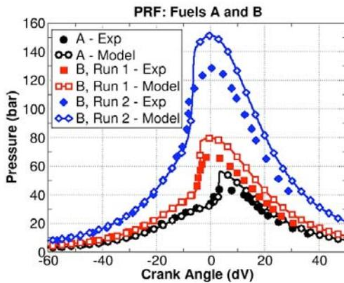
Figure 1: Experimental and simulated pressure curves for fuels A (Run 1) and B (Run 1 and Run 2). Initial temperature and pressure at start of simulations ( $99^\circ$  BTDC) – Fuel A/Run 1: 460 K, 1.2 bar, Fuel B/Run 1: 470 K, 1.7 bar, Fuel B/Run 2: 420 K, 3.2 bar. HCCI engine of Andrae et al. [4].
