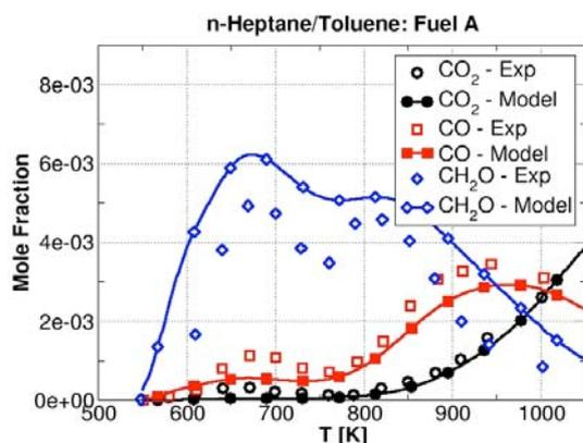
Figure 8: Experimental and simulated mole fractions of  $\text{CO}_2$ , CO and  $\text{CH}_2\text{O}$  as of function of temperature for fuel A. Pressure: 10 bar, Equivalence ratio: 0.2, Residence time=0.5 s. Jet Stirred Reactor of Dubreil et al. [27].
