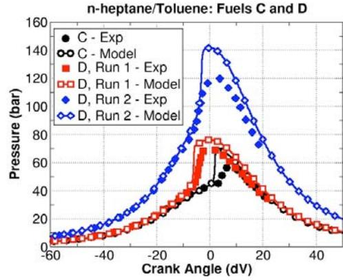
Figure 2: Experimental and simulated pressure curves for fuels C (Run 1) and D (Run 1 and Run 2). Initial temperature and pressure at start of simulations ( $99^\circ$  BTDC) – Fuel C/Run 1: 470 K, 1.6 bar, Fuel D/Run 1: 470 K, 1.6 bar, Fuel D/Run 2: 420 K, 3.1 bar. HCCI engine of Andrae et al. [4].
