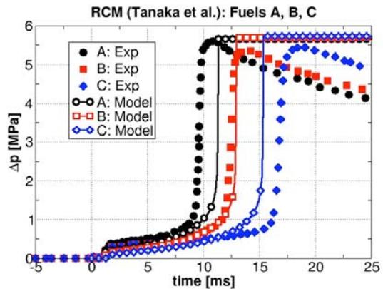
Figure 3: Experimental and simulated pressure change ( $\Delta p$ ) curves for fuels A, B and C. Equivalence ratio: 0.4, Initial temperature: 318 K, Initial pressure: 0.1 MPa, Compression ratio: 16. Rapid Compression Machine of Tanaka et al. [24].
