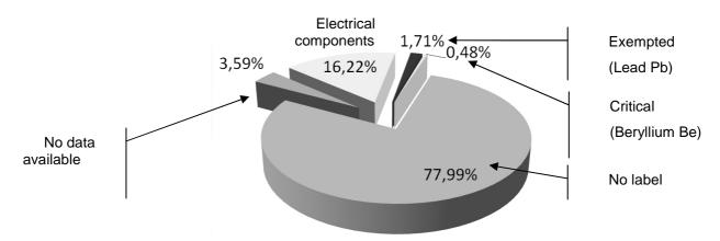
Figure 7: Assessment test results – Materials label repartition quoted on total ECU mass After analyzing Figure 7, it can be concluded that:
