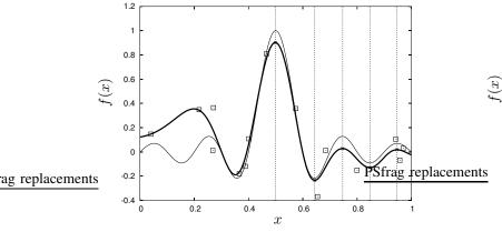
Fig. 3. Approximation (bold solid line) of the sinc function (plain solid line) from noisy observations (squares) taking into account the derivative of the sinc function at positions indicated by the vertical bars.
