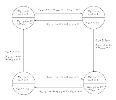
**Fig. 8.** The timed automaton for the C-element  $X_k t$ .
