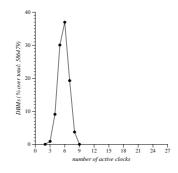
Fig. 15. The distribution of active clocks in an 8-stage STARI.
