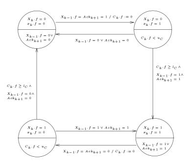
**Fig. 9.** The timed automaton for the C-element  $X_k \cdot f$ .
