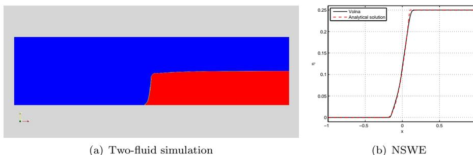
FIGURE 5. Initial deformation of the water column under the gravity force ( $t = 0.2$  s).
