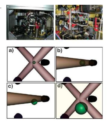
Fig. 4. Up: inside the atom-optics rack (the vacuum chamber and the free-space optics). Down: 3D schematics showing the beams configuration and the interferometer sequence. a) Atom cooling and trapping (MOT, the horizontal retroreflected MOT beam is not shown for clarity), b) First Raman interrogation pulse colinear to the horizontal retroreflected MOT beam, c) second Raman interrogation pulse and d) detection with the MOT beams. The atomic cloud is represented as falling under gravity.
