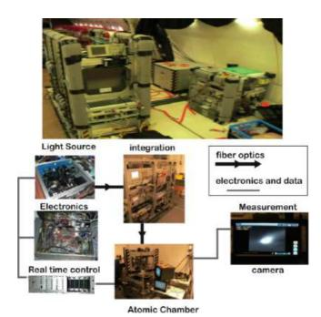
**Fig. 1.** Top: The atom interferometer assembled in the Airbus. The main rack on the left houses the laser sources and the control electronics. The rack on the front right contains the uninterruptable power-supply, the electrical panel and the high-power laser part. The rack on the back right hosts atomoptics part of the experiment. Bottom: the architecture of the atom interferometer.
