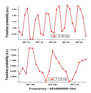
Fig. 6. Optical Ramsey fringes obtained in micro gravity for T=50 ms and T=75 ms, (corresponding to respectively 18 mm and 35 mm of free fall under gravity). The x-axis is the frequency of the Raman transition sideband delivered by the hyperfrequency source and the y-axis represents the non-normalized ratio  $N_2/N$ .
