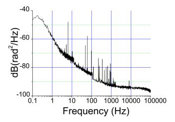
Fig. 2. Spectral density of the phase noise of the quartz recorded by comparison with other ultra-stable quartz oscillators phase-locked on H-Maser of the SYRTE.
