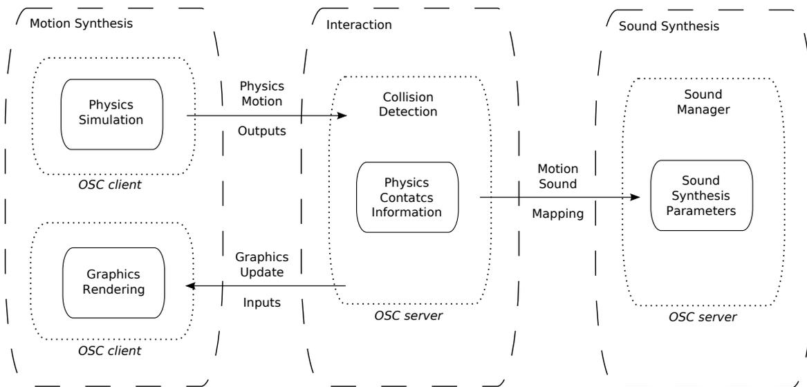
Figure 3: Asynchronous server-client architecture of our system.
