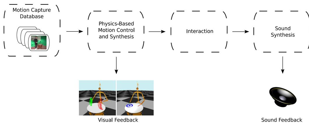
Figure 1: System architecture and multimodal outputs. The *Physics-based Motion Control and Synthesis* step involves a *Motion Capture Database* and results in the *Visual Feedback*. The *Interaction* expresses the mapping between the percussion motion simulation and the *Sound Synthesis*, which results in the *Sound Feedback*.
