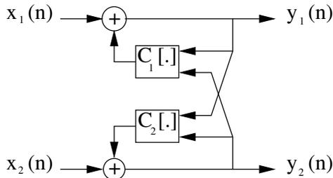
Figure 3: Proposed recurrent network for basic additive-target mixtures.
