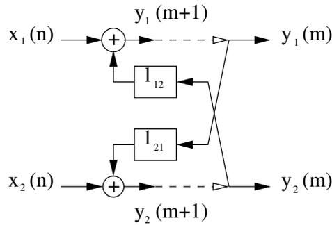
Figure 1: Loop of linear instantaneous recurrent network.
