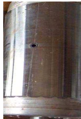
Fig. 10. Rotor with one broken bar.
