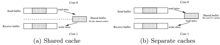
Fig. 1. Performance impact of using a shared buffer: if communicating cores share their cache (a), the additional copy does not lead to a cache miss and therefore causes little overhead compared to a direct copy. On the other hand, if caches are separate (b), significant memory bandwidth is wasted.
