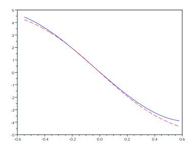
Figure 1: Solid line: estimated drift; dashed line: true drift. The adaptive estimation algorithm on the interval [-0.56, 0.58] selects  $\hat{m} = (0, 3)$ .
