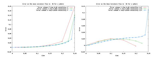
Figure 3: Mean curvature flow problem for different time step and diffusions: scheme 2
