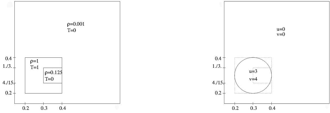
Figure 21. Initial data for test cases Planar geometry (density \rho and temperature T on Left, velocity \mathbf{U}=(u,v) on Right)
