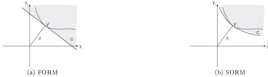
Fig. 5 FORM (a) and SORM (b) method : approximation C of the failure domain D and reliability index \beta
