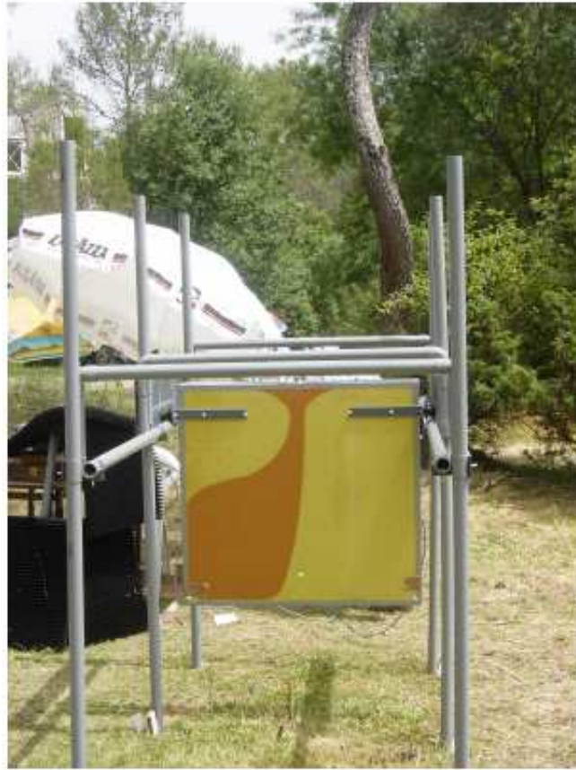
Fig. 16. View of the large-scale exponentially tapered slot antenna mounted on a carriage for test data collection.
