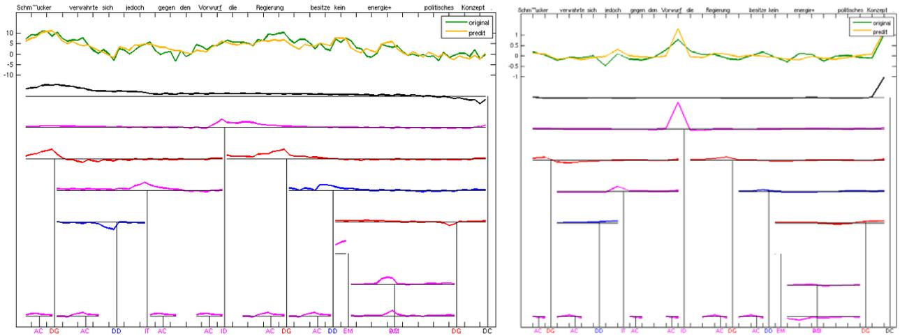
**Figure 1. Comparing original and predicted prosodic contours. Left:  $f_0$ . Right: syllable lengthening. For each caption: top: superposition of predicted (yellow) and original (green) contours; bottom: elementary contours predicted for each discourse function used to encode the linguistic structure of the utterance; the prediction is obtained by superposing and adding these elementary contours. Horizontal axis represents the syllable count**
