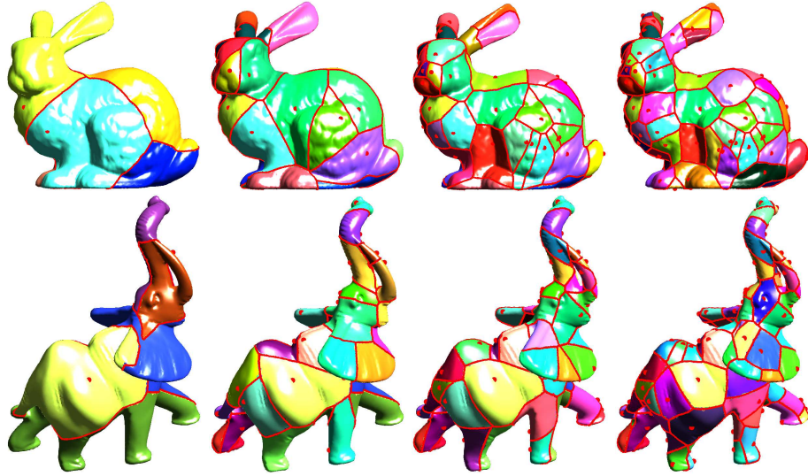
Fig. 21. Example of Voronoi segmentations for an increasing number of seeding points.
