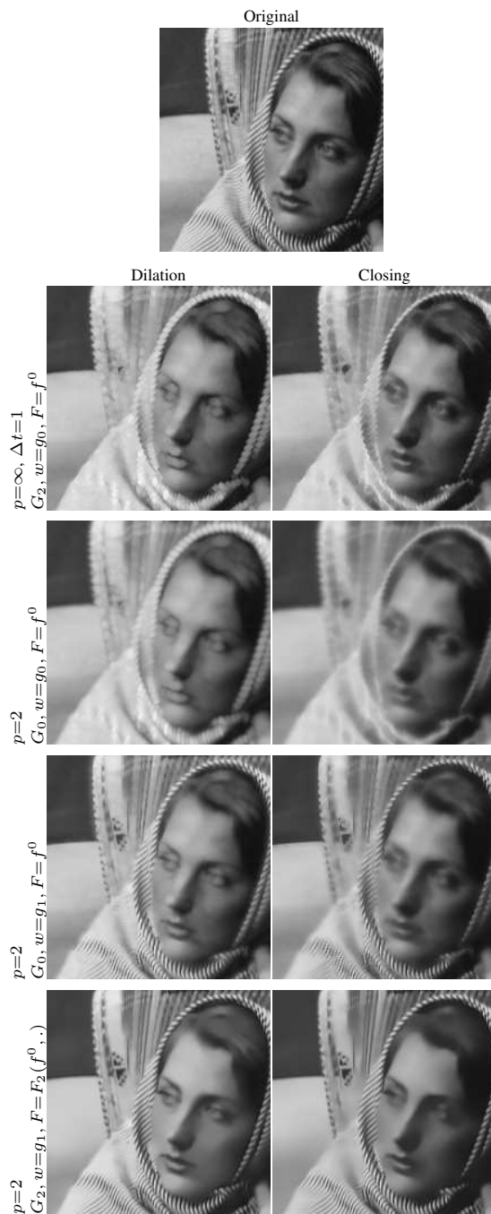
Fig. 2. Adaptive morphological image processing with different p values, weight functions w , graph topologies G , and feature vector F . At top: original image. First and second columns: dilation and closing operations, respectively. First row: algebraic case ( p=\infty, \Delta t=1 ), second row: PDEs case ( p=2 ), third row: weighted case ( w=g_1 ), fourth row: nonlocal patch-based case ( G_2, F_2 ).
