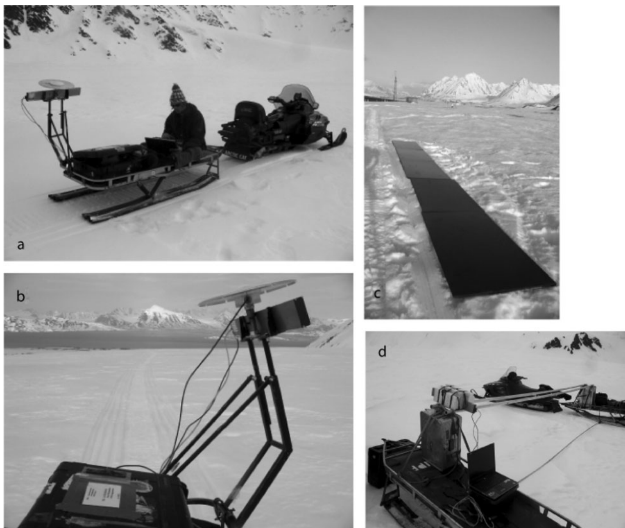
Fig. 1. Pictures of the set-up: (a) general overview of operations; (b) laser and GPS set-up; (c) wooden plate used for the calibration; and (d) laser measurements made on poles.
