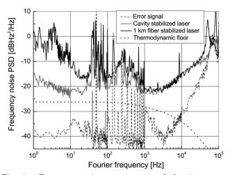
Fig. 3. Frequency-noise power spectral density versus Fourier frequency of the laser stabilized on a 2 km imbalance Michelson interferometer with an antivibration table (dark curve), a reference laser (gray curve), an error signal converted into frequency noise (dashed curve), and a thermodynamic noise floor (dotted curve).
