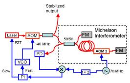
Fig. 1. (Color online) Scheme of the laser frequencynoise-reduction system: AOM, acousto-optic modulator; PD, photodiode; VCO, voltage-controlled oscillator; PI, proportional-integrator filter; FM, Faraday mirror.
