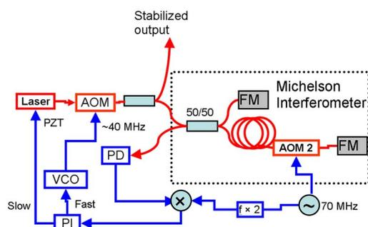
Fig. 1. (Color online) Scheme of the laser frequency-noise-reduction system: AOM, acousto-optic modulator; PD, photodiode; VCO, voltage-controlled oscillator; PI, proportional-integrator filter; FM, Faraday mirror.
