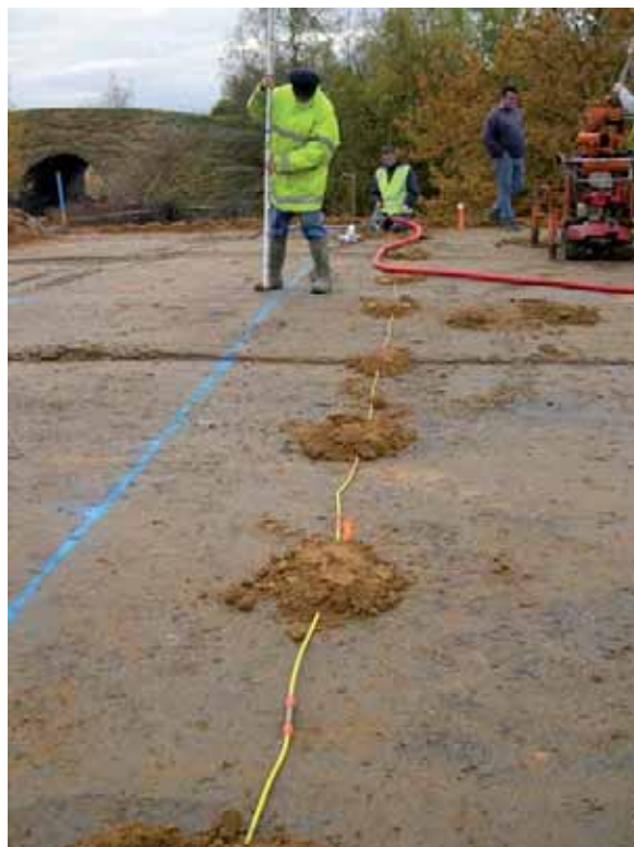
Figure 11 Internal streamer of electrodes for performing electrical resistivity tomography
