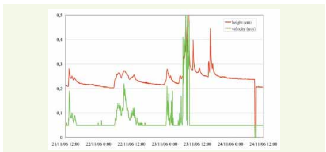
Figure 7 Evolution of velocities and heights in the presence of the V-shaped weir
