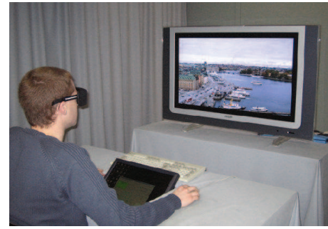
FIGURE 1: Experimental setup: the user is facing the screen with crystal shutter glasses.
