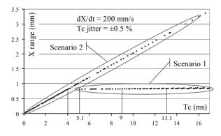
Fig. 9. Conveyor positioning error range.
