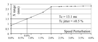
Fig. 10. Effect of conveyor speed perturbation.
