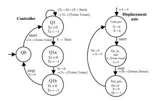
Fig. 5. Hybrid automata of the axis control.
