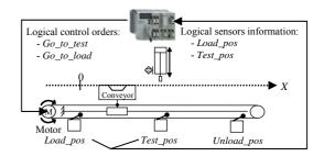
Fig. 4. Displacement axis of station 2.
