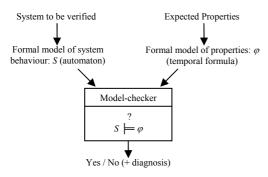
Fig. 1. Model-checking scheme.
