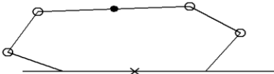
(b) Double support (half step n ): The projection of the platform center is closer to the back leg tip
