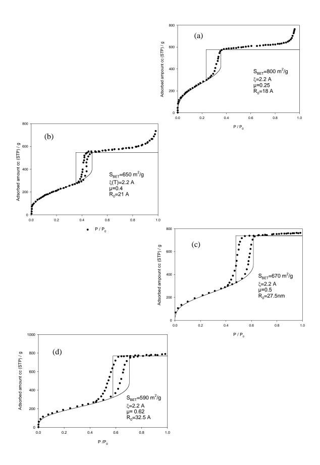
Figure 7: Ar adsorption at 87 K in various MCM type pores (a-d) comparison with experiment (points), model (lines)
