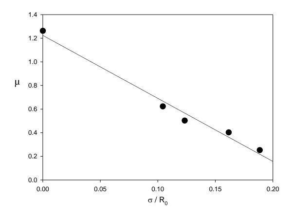
**Figure 8**: μ exponent in equation (22) as a function of the reciprocal of the pore size. The line is a linear regression.
