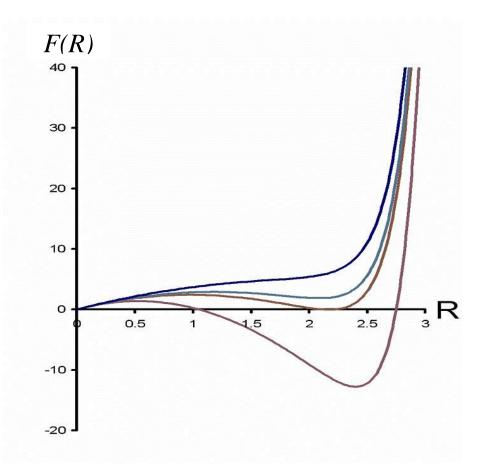
**Figure 4.** F(R) at constant temperature *T* for increasing pressures of the gas phase,  $P_V$  (*from bottom to top*). The core radius *R* is in nm, the grand free energy  $\Omega$  is in  $10^{-19}$  J (see text).
