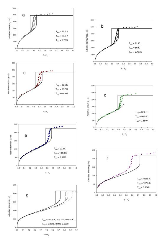
**Figure 5**: Ar adsorption isotherm in a 4.2 nm diameter pore at various temperatures. (a-f) comparison with experiment (points), model (lines), (g) calculated isotherms as the temperature approaches  $T_{cc}$ . Experiment and model are plotted at equal T/T<sub>cc</sub> ratio.
