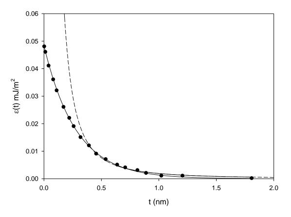
**Figure 2.** Evolution of the coupling parameter  $\varepsilon(t)$  as a function of the adsorbed film thickness *t* for argon at 87 K,  $\rho_L = 1.394$  g/cm<sup>3</sup>, using  $\varepsilon(t) = \exp\left(-\frac{t}{\xi(T)}\right)$  as a fitting function with  $\xi(T) = 0.278$  nm (solid line); using  $\varepsilon(t) = A/t^2$  with  $A = 1.896 \ 10^{-3} \text{ mJ/m}^2$ .
