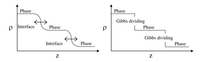
**Figure 1.** (*left*) A real system is composed of three phases 1, 2, and 3 separated by two interfaces 1/2 and 2/3. (*Right*) Using the Gibbs surface dividing theory, the system is modelled as three homogeneous phases separated by infinitely thin, fictive interfaces that are located in the middle of the real interfaces.
