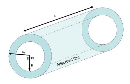
**Figure 3.** Schematic view of the cross section of a cylindrical pore of radius  $R_0$  (adsorbent) showing the equilibrium between an adsorbed film at the pore surface and the gas phase in the pore center. The thickness of the adsorbed film is  $t = R_0 - R$ .
