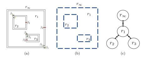
Figure 3: The three different models composing a topological map. (a) A 2-map representing the topology with darts and  $\beta_i$  relationships; (b) A geometrical matrix that points out active linels and pointels; corresponding elements are linked together (for visibility reasons, dotted lines represent only up/down relations between regions); (c) A tree of regions for inclusion relations.
