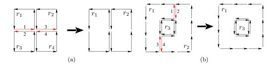
Figure 9: Configurations encountered during the merging operation between two adjacent regions. (a) Simple adjacency between  $(r_1, r_3)$  and  $(r_2, r_4)$ : the corresponding edges (1, 2) and (3, 4) are removed if the merging criterion is verified; (b) Multiadjacency between  $(r_1, r_2)$ : if (1, 2) has been removed, (3, 4) is removed independently of the merging criterion.
