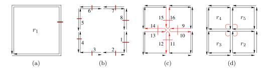
Figure 6: Decomposition in four steps of the splitting process applied on a region  $r_1$  enclosing four pixels. (a) Initial region; (b) Splitting edges: darts 1 to 8 are stored into *list* (external border of  $r_1$ ); (c) Insertion of 4 dangling edges while testing darts 1, 3, 5 and 7; (d) Sewing correctly dangling edges while testing darts 9 and 13.
