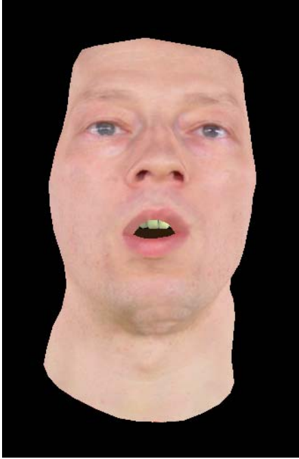
Figure 1: Synthetic display generated from a mesh of the 398 marker positions and 30 points of an additional lip model, rendered with a static cylindrical texture.
