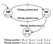
Fig. 6. State machine for the formalization of PROP5
