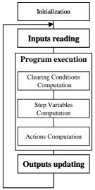
Fig. 3. Cyclic scan monitor of the PLC
