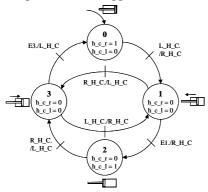
Fig. 8. Horizontal movement model
