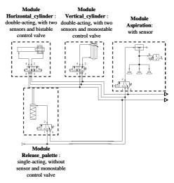
Fig. 7. Modular plant decomposition
