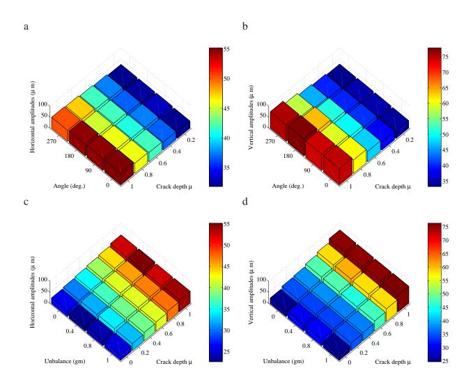
Figure 10: Evolutions of the  $2 \times$  maximum amplitudes at one-half of the first critical speed for the horizontal and vertical directions at the plane 2 (a,b) versus the slot depth and the phase between the unbalance and the slot front for an unbalance of 0.4gm (c,d) versus the slot depth and the unbalance with a phase between the unbalance and the slot front of 0 deg.
