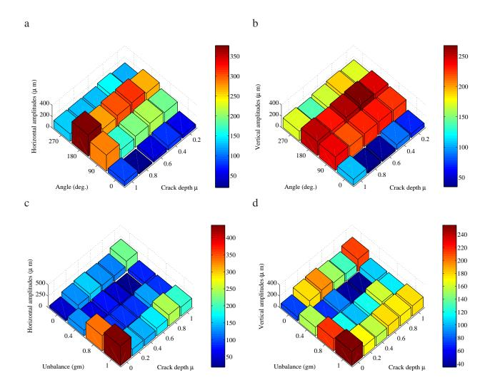
Figure 9: Evolutions of the  $1 \times$  maximum amplitudes at the first critical speed for the horizontal and vertical directions at the plane 2 (a,b) versus the slot depth and the phase between the unbalance and the slot front for an unbalance of 0.4gm (c,d) versus the slot depth and the unbalance with a phase between the unbalance and the slot front of 0 deg.
