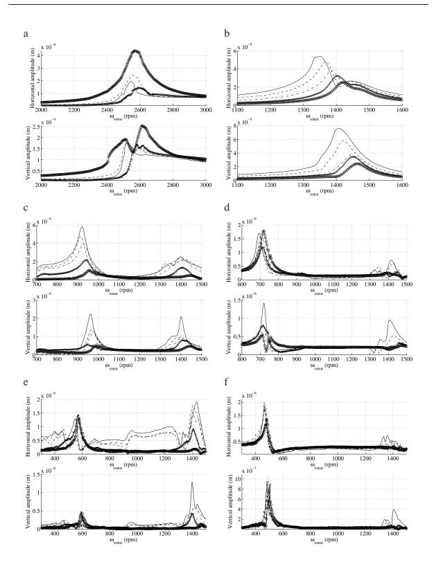
Figure 8: Evolutions of the  $n \times$  amplitudes for various crack depths with an unbalance of 1gm and a phase between the unbalance and the slot front of 0 deg. (a)  $1 \times$  - plane A2, (b)  $2 \times$  - plane A2, (c)  $3 \times$  - plane A1, (d)  $4 \times$  - plane A3, (e)  $5 \times$  - plane A1, (f)  $6 \times$  - plane A3 (-o- uncracked, -+-  $\mu = 0.2$ , -.-  $\mu = 0.4$ ,  $\cdots \mu = 0.6$ , --  $\mu = 0.8$ ,  $-\mu = 1$ )
