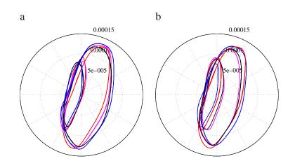
Figure 14: Changes in the orbital patterns at the one-half of the first critical speed as a function of (a) the phase with  $\mu = 1$  and an unbalance of 1gm (red: 0 deg., magenta: 90 deg., blue: 180 deg., black: 270 deg.), (b) the unbalance with  $\mu = 1$  and a phase of 0 deg. (black: 0gm, blue: 0.4gm, magenta: 0.8gm, red: 1gm)
