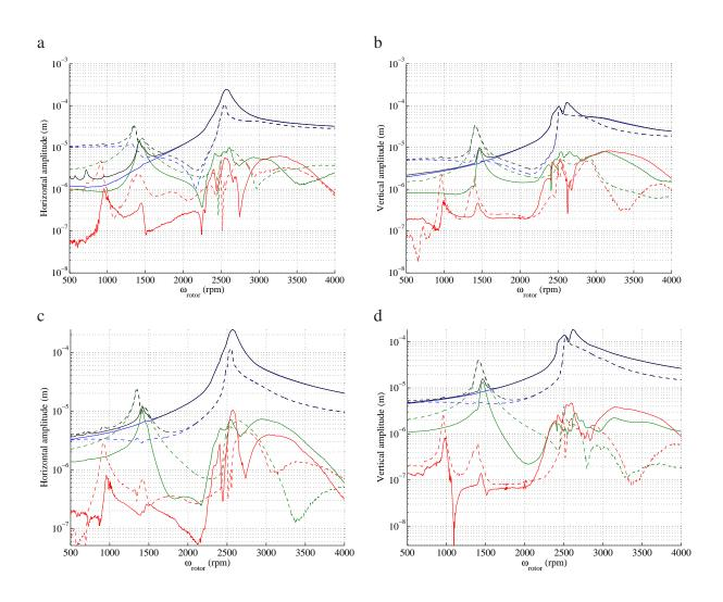
Figure 4: Evolution of the global response,  $1 \times$ ,  $2 \times$  and  $3 \times$  amplitudes for the healthy and slooted rotors ( $\mu = 1$ ) with an unbalance of 1gm and a phase between the unbalance and the crack front of 0 degree. (a-b) plane A1 (c-d) plane A3 (solid lines = uncracked rotor, dashed lines = cracked rotor, black = global amplitudes, blue =  $1 \times$ , green=  $2 \times$ , red =  $3 \times$ )
