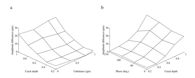
Figure 11: Differences between the horizontal and vertical directions of the  $2 \times$  maximum amplitudes at one-half of the first critical speed on plane A2 (a) for various crack depths and unbalance with a phase of 0 deg. (b) for various crack depths and phases between the unbalance and the crack front with an unbalance of 0.4gm
