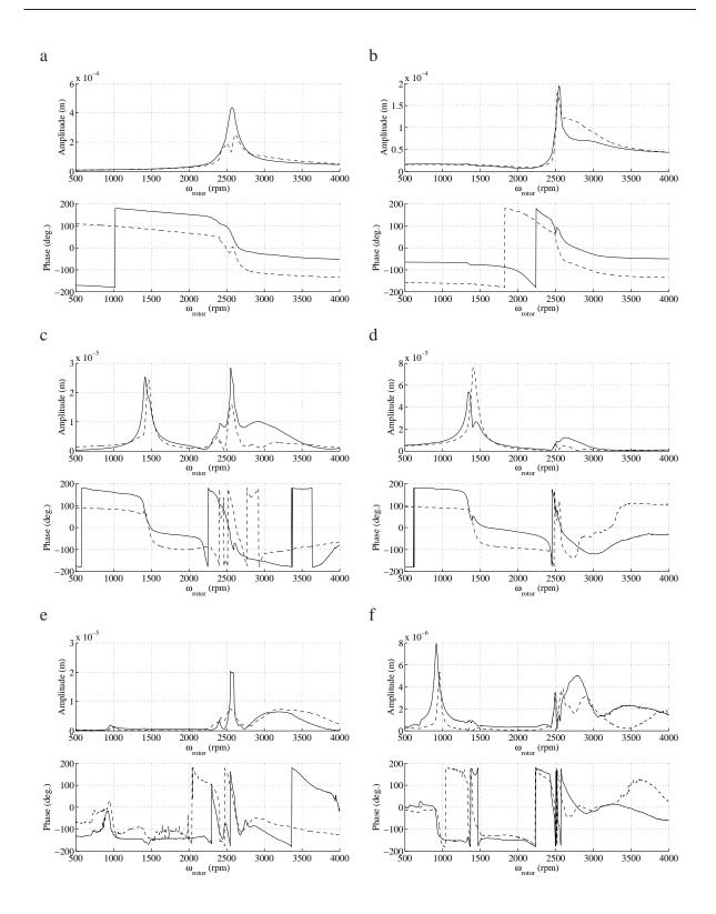
Figure 3: Evolution of  $n \times$  amplitudes and phase in plane A2 for the healthy and slotted rotors  $(\mu = 1)$  with the unbalance of 1gm at 0deg. (a)  $1 \times$ , healthy rotor (b)  $1 \times$ , slotted rotor (c)  $2 \times$ , healthy rotor (d)  $2 \times$ , slotted rotor (e)  $3 \times$ , healthy rotor (f)  $3 \times$  slotted rotor (solid lines = horizontal direction, dashed lines = vertical direction)
