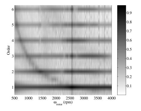
Figure 6: Evolutions of the  $n^{th}$  orders for the healthy rotor with an unbalance of 1gm and a phase between the unbalance and the crack front of 0 deg.
