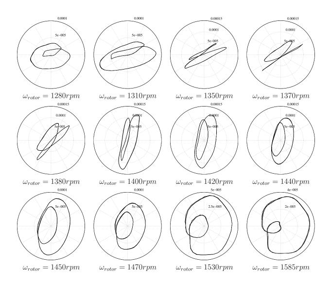
Figure 12: Orbital evolutions of the cracked rotor for plane A2(with  $\mu = 1$ ) around one-half of the first critical speed with an unbalance of 1gm and a phase between the unbalance and the crack front of 0 deg.
