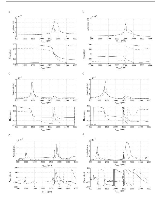
Figure 2: Evolution of  $n \times$  amplitudes and phase in plane A2 for the healthy and slotted rotors ( $\mu = 1$ ) with the initial residual unbalance (a) 1×, healthy rotor (b) 1×, slotted rotor (c) 2×, healthy rotor (d) 2×, slotted rotor (e) 3×, healthy rotor (f) 3× slotted rotor (solid lines = horizontal direction, dashed lines = vertical direction)
