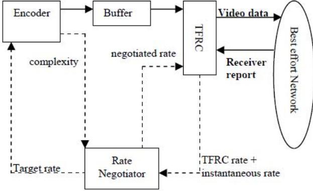
Fig. 1. The VTFRC architecture.
