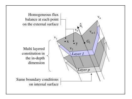
Figure 1. Illustration of the multi-layered in-depth composition of an element and the homogeneity with respect to boundary conditions on the internal and external surfaces.
