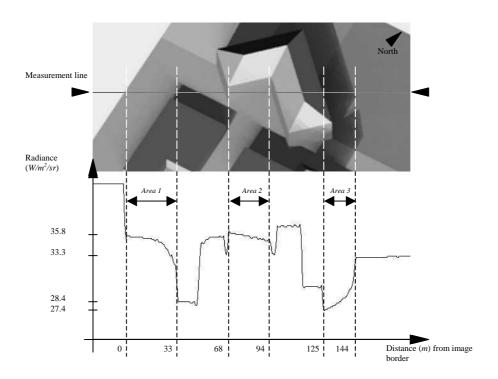
Figure 4. Radiance profile along the measurement line at 11:00 am – band III.
