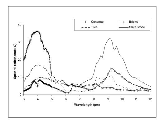
Figure 6. Spectral reflectance variations of materials used in the simulation between 3 and 12  $\mu m.\,$
