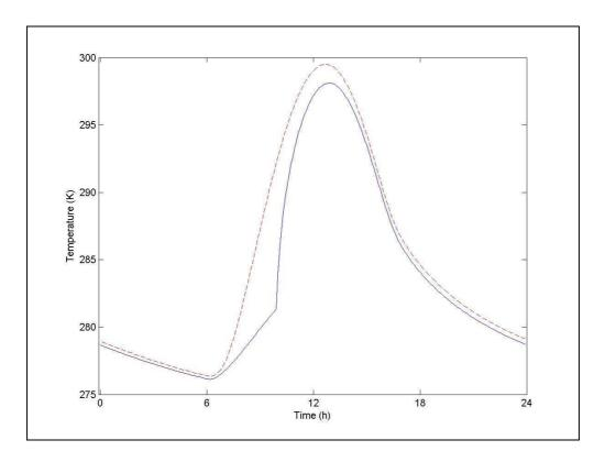
Figure 5. Daily profile of surface temperature (in Kelvin). In dashed line, temperature of an object sunlit all the day long. In solid line, temperature of an object shadowed from sunrise to 10:00 am.
