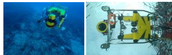
Figure 2: The ROV in the water with digital camera and flash lights in their housing; left: side view of the ROV; right: view from the seabed upward. The flash lights are on the side of the camera
