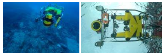
Figure 2: The ROV in the water with digital camera and flash lights in their housing; left: side view of the ROV; right: view from the seabed upward. The flash lights are on the side of the camera
